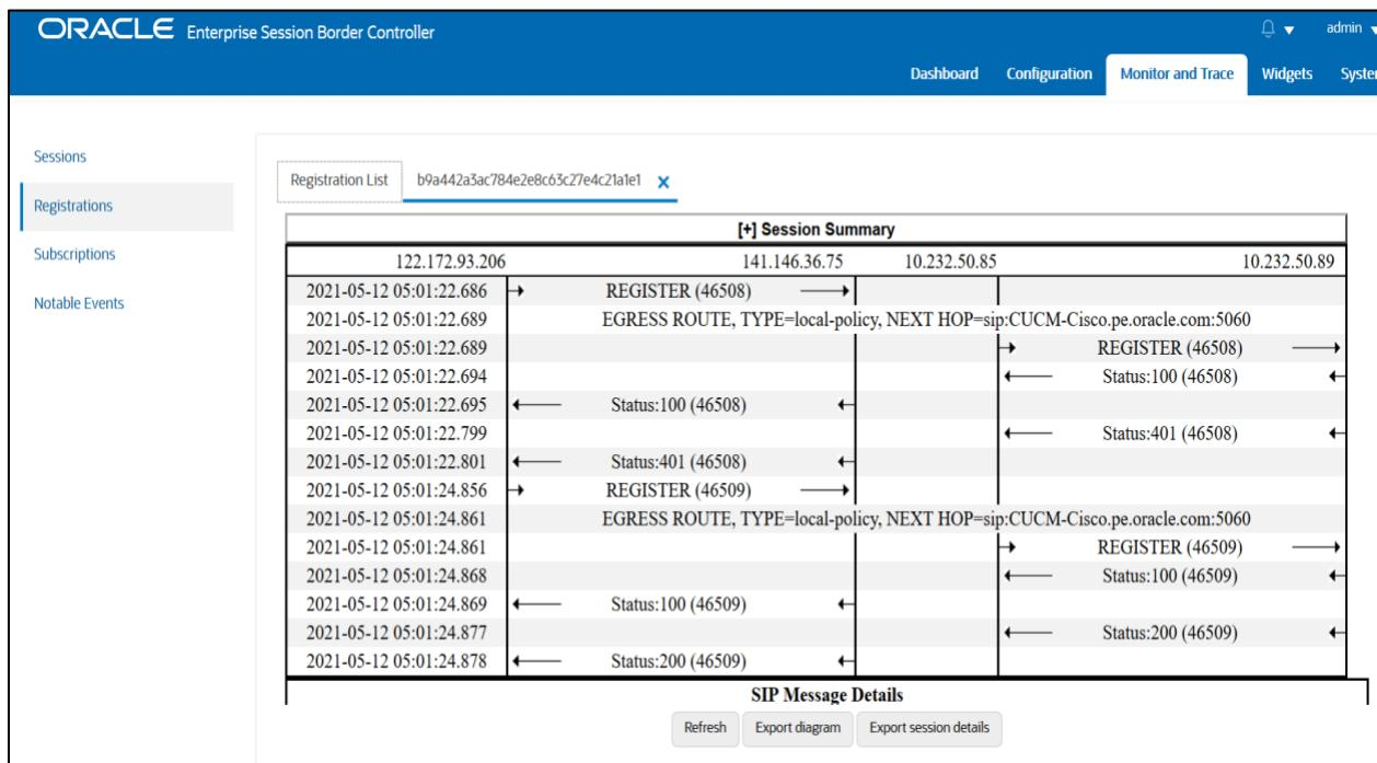
3. Make Call from Cisco Remote user to the Twilio Elastic Sip Trunk user and check the call flow. Now, there will be 2 call legs (hair pinned call) as the call reaches Cisco CUCM first and then reaches Twilio trunk user after that as given below.
