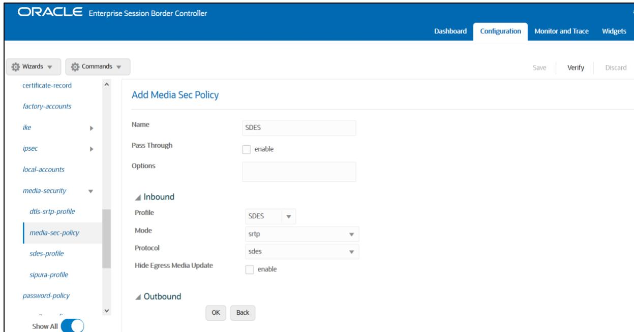
Similarly, Create Media Sec policy with name RTP to convert srtp to rtp for the Cisco side which will use only TCP/UDP as transport protocol. **Assign this media policy to the Cisco Realm.**
