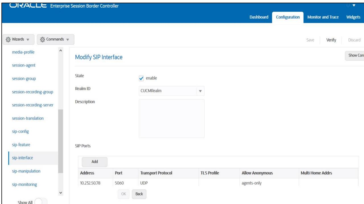
Once sip-interface is configured – the SBC is ready to accept traffic on the allocated IP address.
